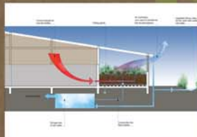
Green filter design for air purification 7200m 2 /hour is treated to 0.5m 3 of green filter depth Zero input of polluted air into the atmosphere - 2008
