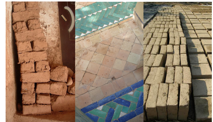
Earth and "Bejmat" construction materials
