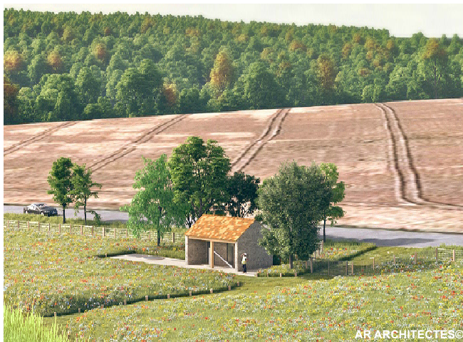
Bioclimatic architecture in timber frame, stone cladding and tiles.
